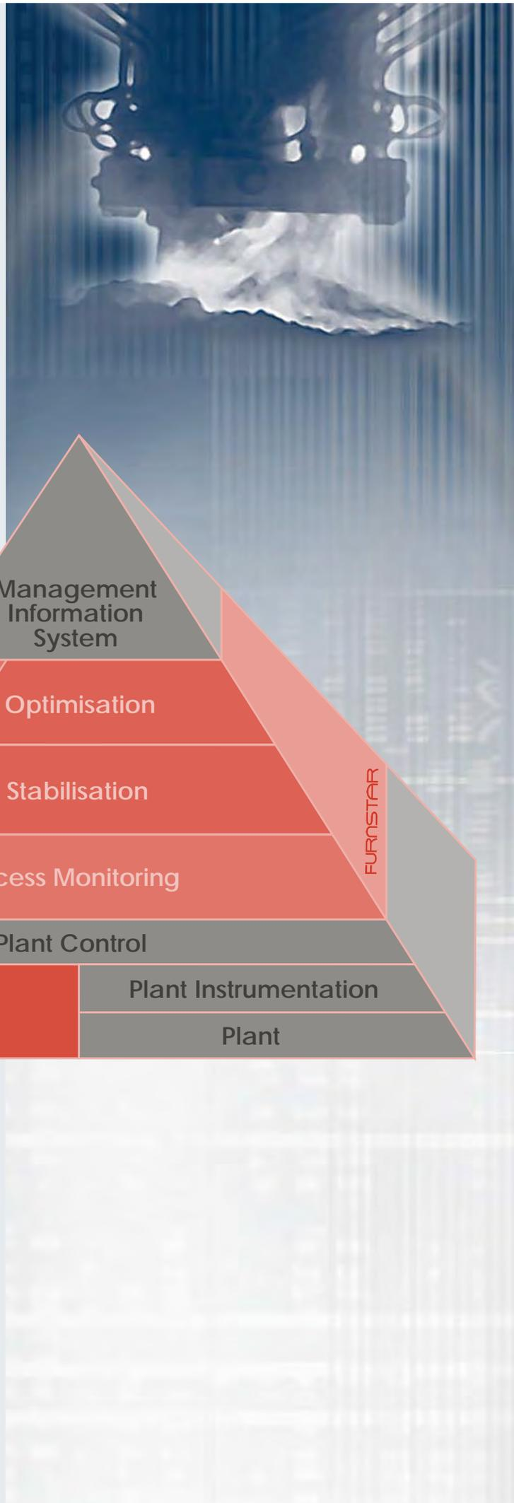
FurnStar Minstral is a submerged-arc furnace control system that optimises furnace operation by means of a patented resistance algorithm, enabling stable operation at optimal power.
