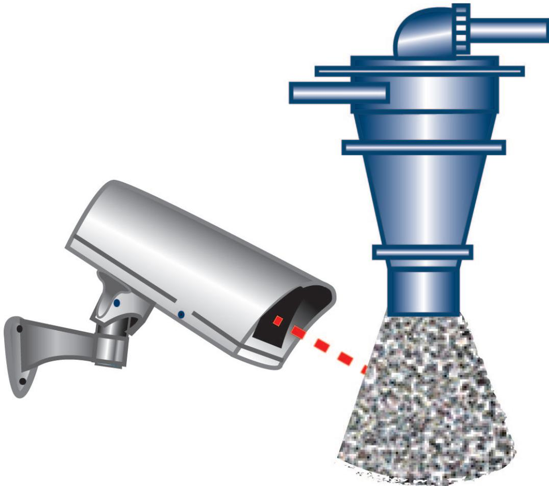
The hydrocyclone classifier forms an integral part of the milling circuit. The overall performance of the milling circuit depends directly on the performance of the hydrocyclone classifier. Plant operators have traditionally used the shape of the hydrocyclone underflow to assess the overall efficiency of the milling circuit – the CyLas provides this information on-line.
